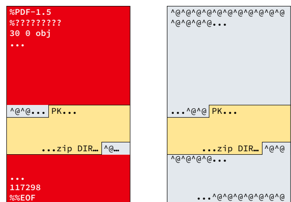
Figure 2: Padding the zip with ininflatable bags of null characters solves the issue illustrated in Figure 1 by ensuring that the detached zip has the same offsets as the polyglot.
