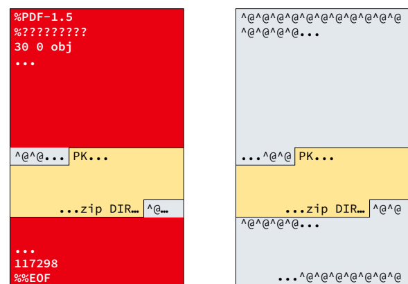
Figure 2: Padding the zip with inflatable bags of null characters solves the issue illustrated in Figure 1 by ensuring that the detached zip has the same offsets as the polyglot.
