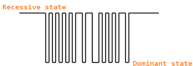
Physically, communication frame on a bus is a voltage waveform – in fact, it is much longer than presented here
